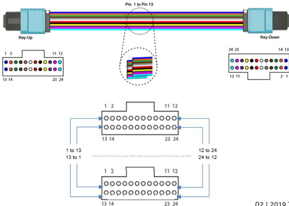
By creating a diagram of a channel with the component type symbol marked at each component, including cables, cords, and adapters, and considering their effect along the length of the channel, you can predict the polarity outcome and determine operability. The designer would strive to ensure that there are an odd number of transpositions of the same type across the channel so that Tx goes to Rx from end to end.
