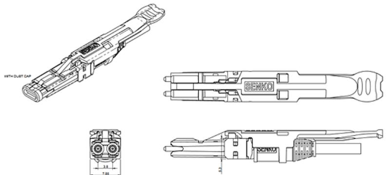
**Bottom Line:** The new CS® connector will offer an unparalleled level density for next generation data centers with the latching mechanism making it easier to manage individual connections as well as support 400G Ethernet through the double duplex connection (two CS connectors side by side) in the 2X200Gig QSFP-DD/OSFP transceivers.
