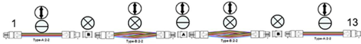
In this example there are four Type B devices which would result in no transposition of Tx and Rx since there are an even number of them. But there are five row transposition devices, which would result in a having the top and bottom row fibers transposed and therefore this system would function properly supporting 100G-SR10 channels.
